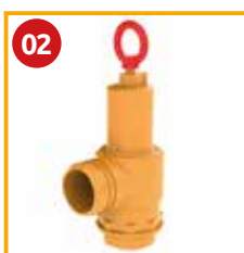
Overpressure Safety Valve - 2" Code 5100200011 Setting range: +0,3 bar / +1,5 bar Working temperature: -20°C / +90°C Thread: G 2" Weight: 1,2 kg
